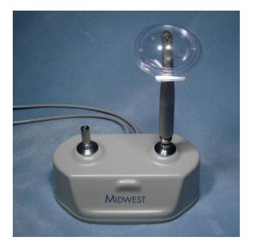
Run handpiece without bur using handpiece hose or Midwest Air Station. Run for 30 seconds or until normal speed is reached and all excess cleaner/lube is expelled.
