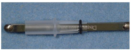
5. Push tool up until the fingers reach the groove
