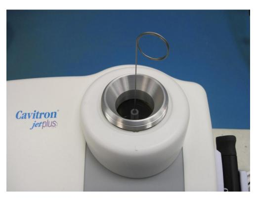
If strong airflow is not heard or felt from the powder bowl center tube, J nozzle may be clogged. Insert the JET-Mate cleaning wire [81075] into the powder bowl center tube down into the small hole in the J nozzle to clear the clog.
